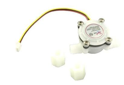
This water flow sensor is basically a small turbine whose output signal is a series of digital pulses. The frequency of the pulses is proportional to the flow rate of the liquid passing through the sensor. That digital signal, whose frequency is in the range between 0Hz and 100Hz, can be read directly through one of the digital input/output pins of a microcontroller.
